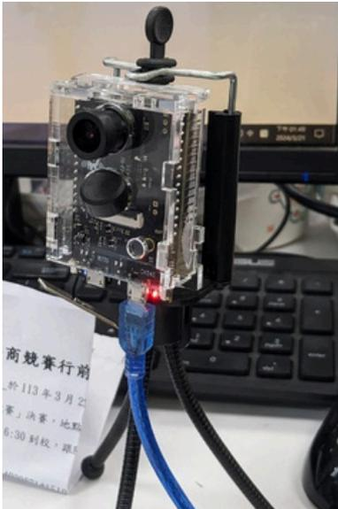
The AMB82 mini development board can be connected to various electronic components such as LEDs, switches, pressure sensors, humidity sensors, and PM2.5 dust sensors. The collected data can be uploaded via WiFi for use by applications, enabling the realization of IoT applications.
